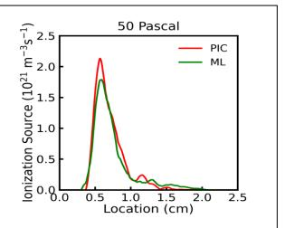
**Fig. 1**. Comparison of directly measured ionization rates from a PIC simulation compared to the values predicted with machine learning based on local plasma conditions.
